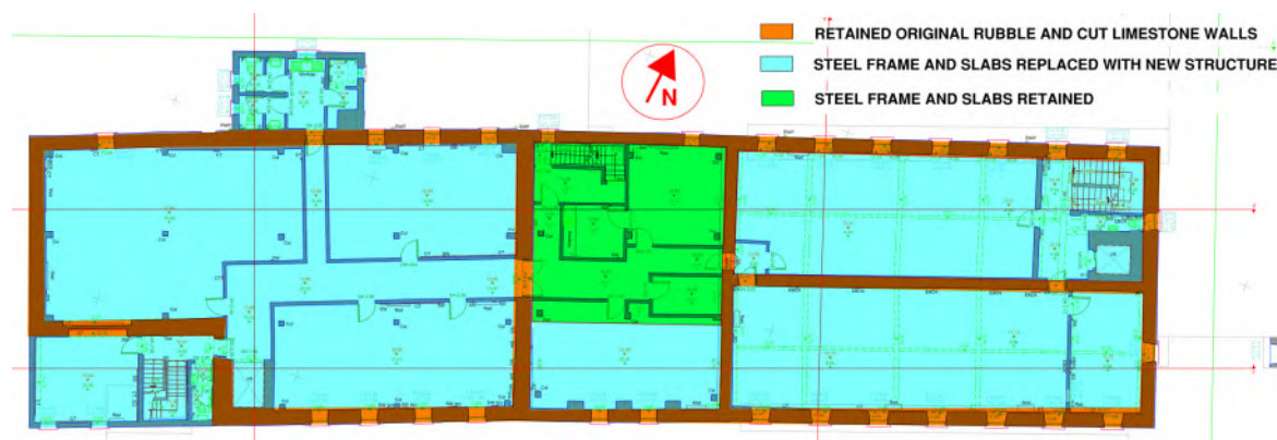
Figure 4.2 Level 1 structural interventions
