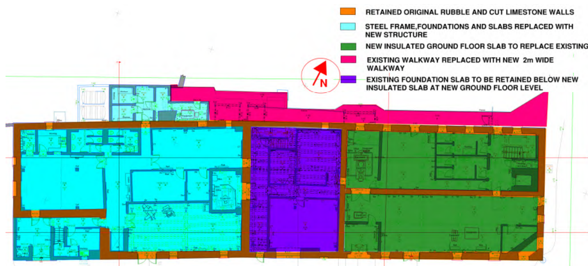
Figure 4.1 Ground floor structural interventions
